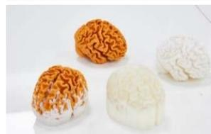
Brain model produced by Ricoh 3D printer
